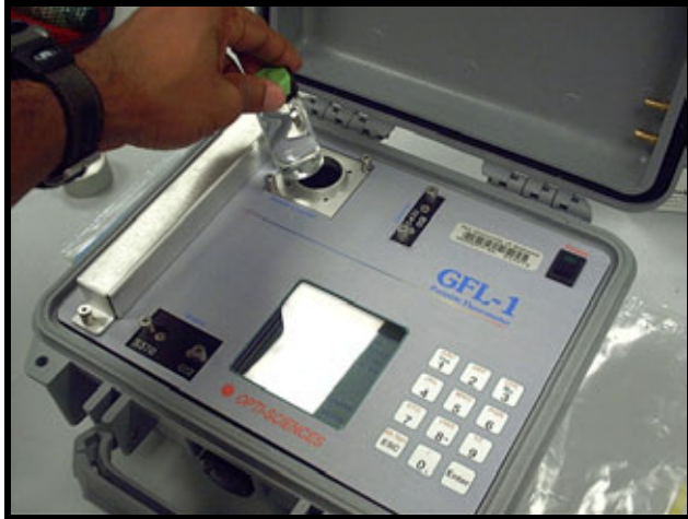
Figure F3.5: Placing Sample into Sample Chamber
