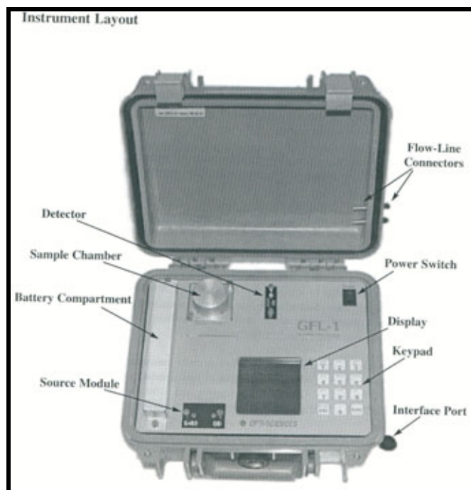
Figure F3.2: GFL-1 Portable Field Fluorometer
